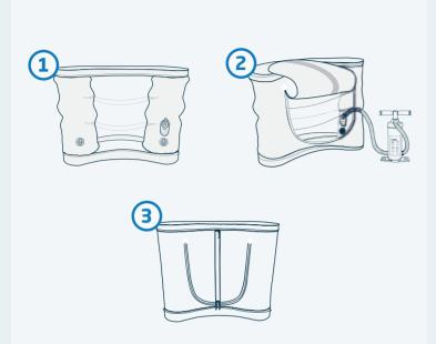
The GYBE® Counter is built up in just three steps: Attach the pump hose into the inflation valve, fill the struts and the counter will be ready.
