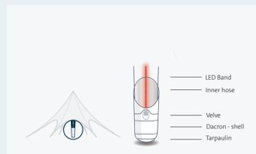
The inflatable supporting structure is built-up in just a few minutes.
