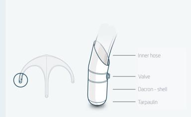
The inflatable supporting structure consists of a high-strength Dacron-shell.
